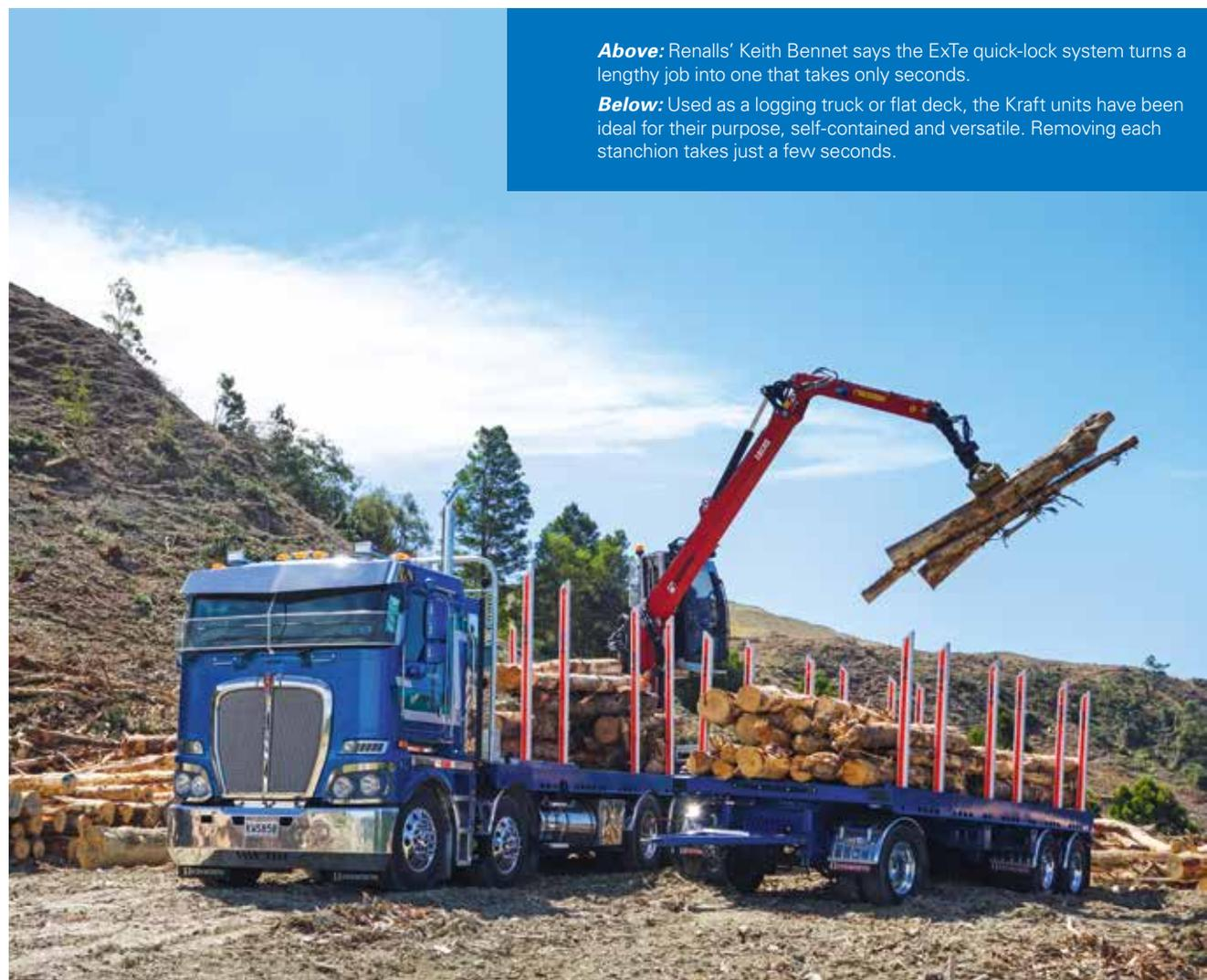
**Above:** Renalls' Keith Bennet says the ExTe quick-lock system turns a lengthy job into one that takes only seconds.
